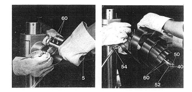
Replacing the steel cable of the baseboard servo-adjustment
